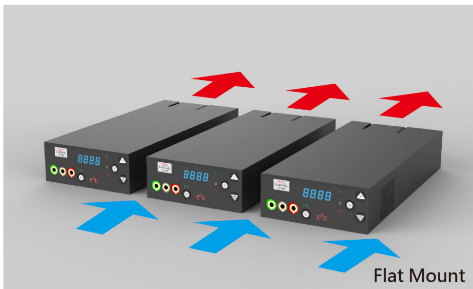
Illustration for the flat mount and the associated ventilation flows
